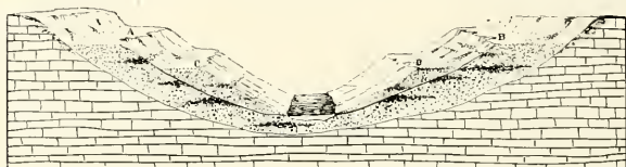
FIG. 28. Diagram showing two sets of terraces developed from aggradational flats.
